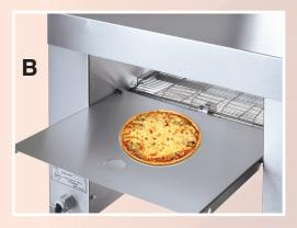
When we want to toast products such as pizza, big baguette, burger etc, the door should be opened, as it is shown in picture B, and based on specific holders
